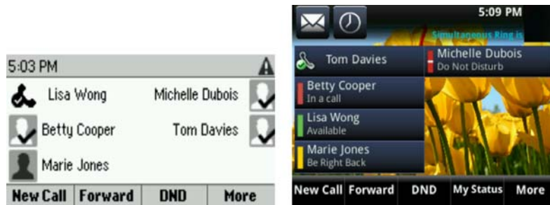
Favorite Skype for Business contacts on the Lines screen on VVX 300 series and VVX 500 series phones
